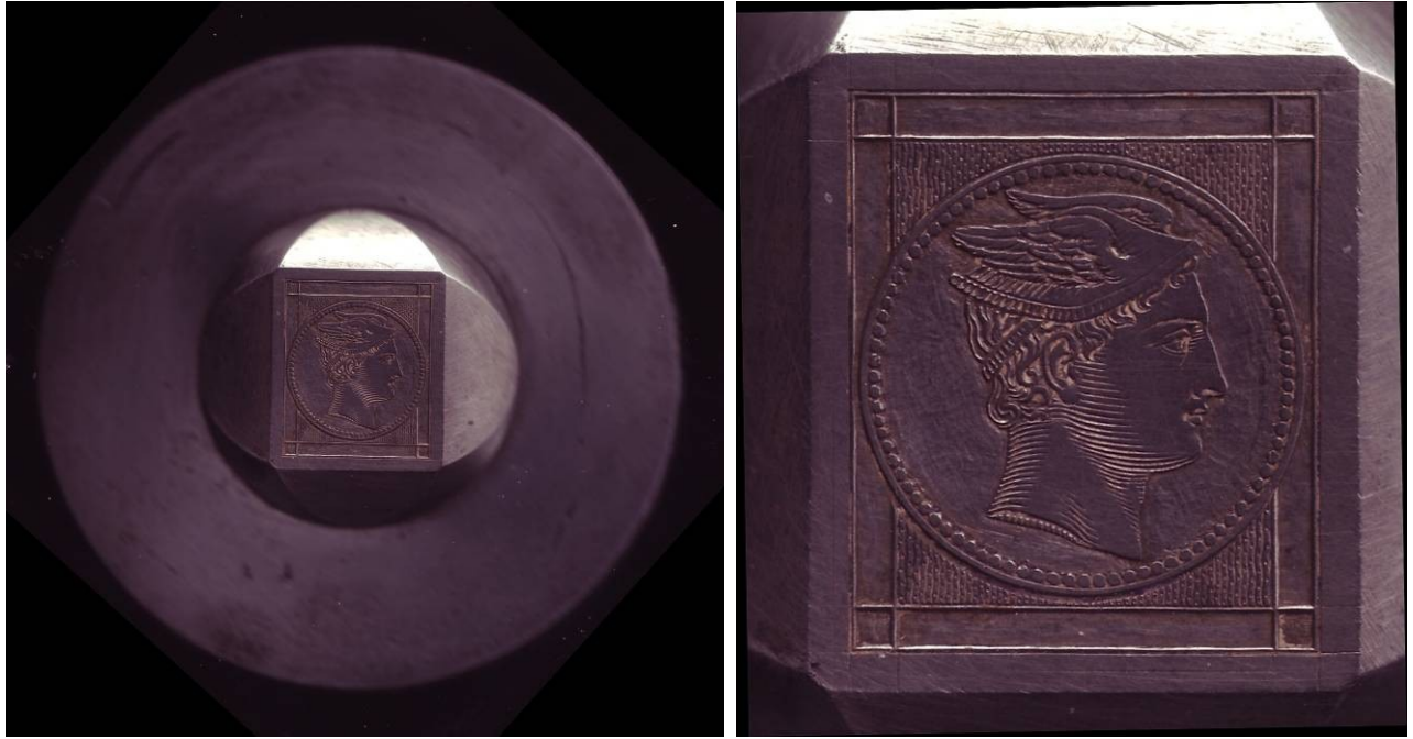
Figure 7: The provisional punch of the "Large Hermes Head".
